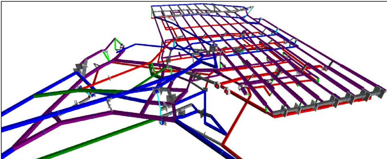
Fig.2. Ventilation network model/diagram of large metal mine (VnetPC program)
