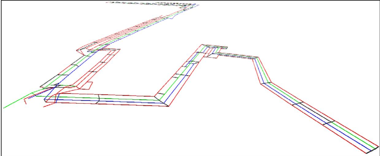
Fig.1. Ventilation network model/diagram of small coal mine (VnetPC program)
