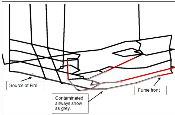
Fig. 3. Fire simulation graphical design view (MineFire program)
