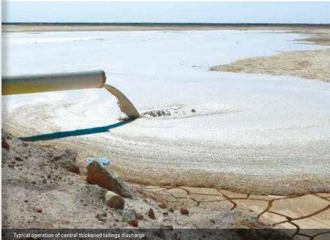
Typical operation of central thickened tailings discharge
