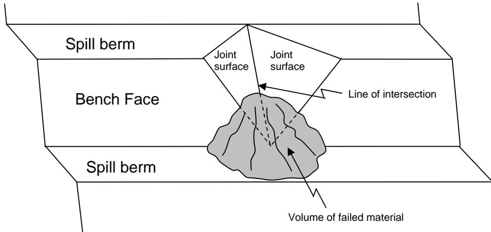
**Figure 2: 3-D illustration of wedge failure**
