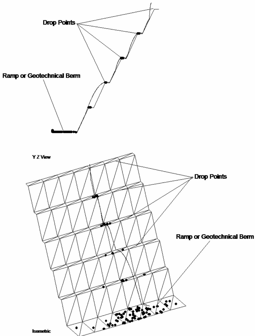
Figure 19: Typical rock fall analysis showing the drop points and the pit ramp or geotechnical safety berm
