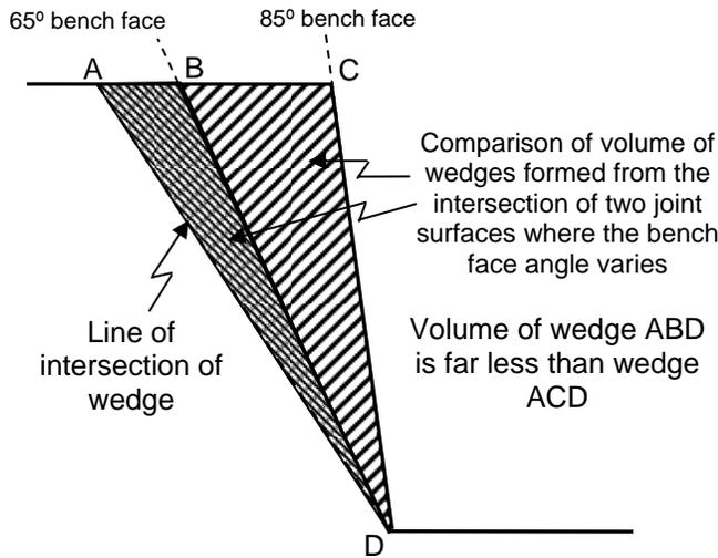
**Figure 7: Sectional illustration of the importance of bench face geometry in determining wedge volume**
