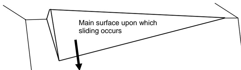
**Figure 3: 3-D illustration of failure of a highly asymmetric wedge approximating planar failure**
