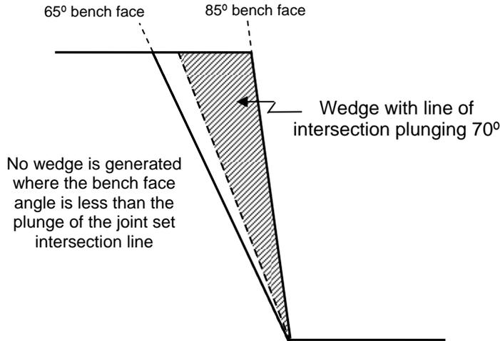
**Figure 6: Sectional illustration of the importance of bench face geometry and joint line of intersection in wedge generation**
