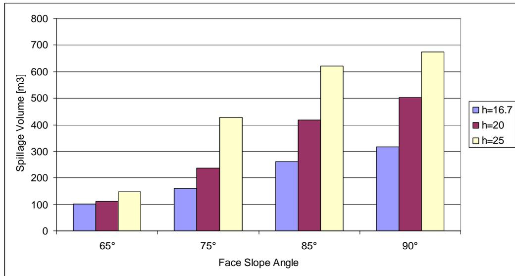
**Figure 18: BSA=58°. Average spillage volume per wedge**
