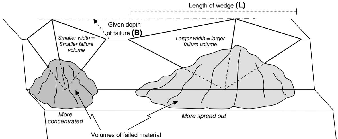
**Figure 9: 3-D illustration of wedge shapes and distribution of failure volumes**
