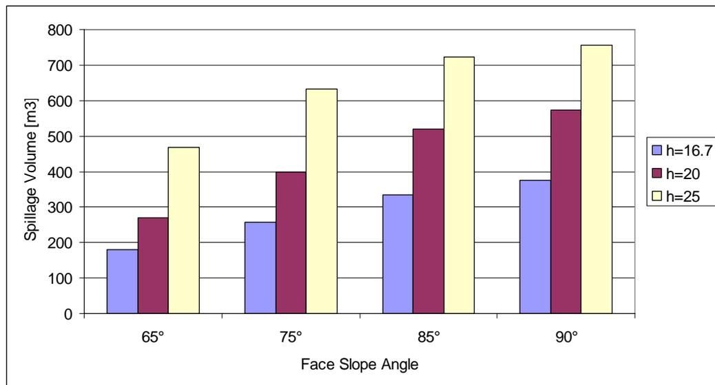
**Figure 16: BSA=46°. Average spillage volume per wedge**
