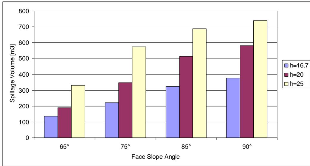
**Figure 17: BSA=52°. Average spillage volume per wedge**
