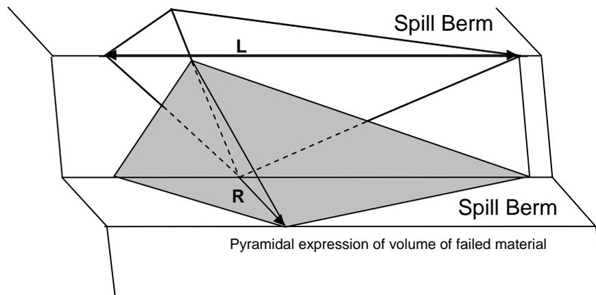
**Figure 12: 3-D illustration of the pyramidal distribution of failed material on a spill berm**
