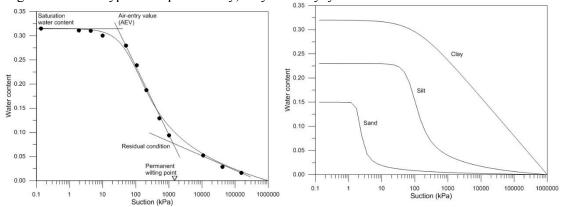
Figure 1. SWCC Example (Left). Typical Shape of sandy, silty and clayey soils (Right).
