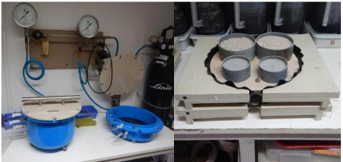
Figure 4. Pressure plate equipment used to obtain SWCC
