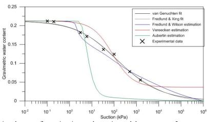
Figure 7. Comparison between fits, estimations and experimental data, spent ore 3.
