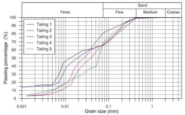
Figure 2. Particle size distribution of tailings.
