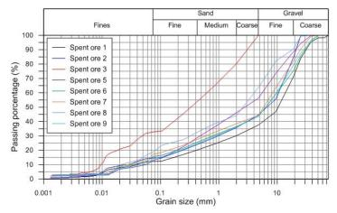
Figure 3. Particle size distribution of spent ore
